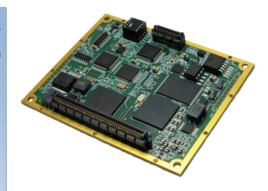
TMCORE02 from TEMAI Ingenieros is a computing and controller platform based on 32 bit Freescale Coldfire Microcontroller at 250MHz and Altera MaxII CPLD enhanced from TMCORE01 platform for aero products under DAL A and DAL B certification for control / monitor architectures with isolated/non isolated power and signals configuration, manufactured under IPC600 and IPC610 class 3.
