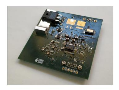
HDVDC SSPC from TEMAI is a Power Contactor based on Solid State technology. Silicon Carbide (SiC) MOSFETs are used in order to operate at high voltage (over 270VDC) and to reduce the conduction resistance ( $R_{DSON}$ ).
