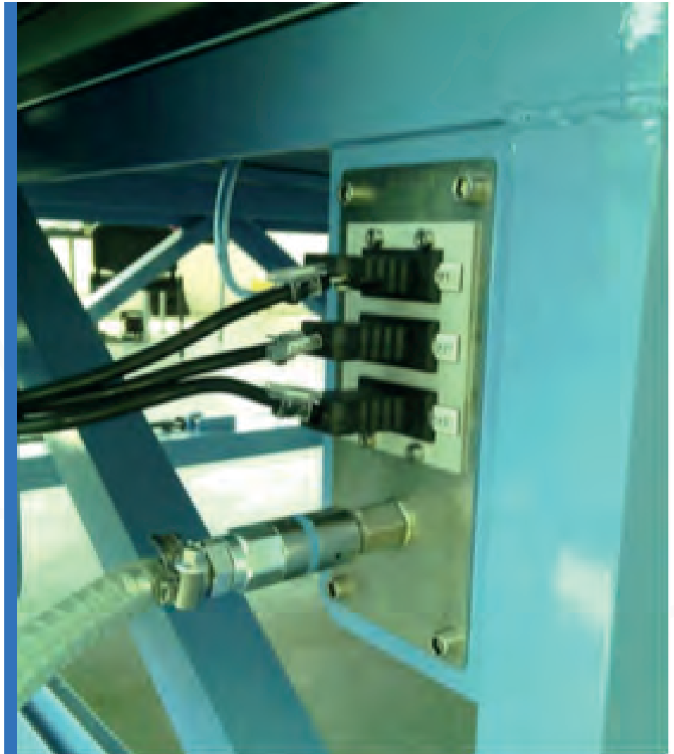
Fig 2. Connecting plate for Thermocouples and Vacuum line
